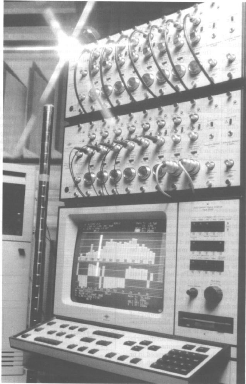
Fig. 1 Multichannel Analysis System 3550 comprising an analyser and two data acquisition units each containing 8 input modules
